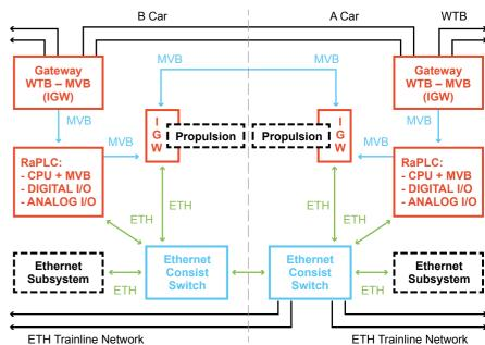
event recorders. Delivery includes a gateway to the propulsion system from Toyo Denki.
